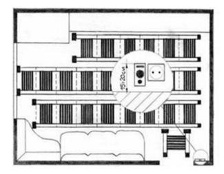
Leave a space and padding around the perimeter of the room size from 4"-15"(10 to 40 cm) spacing between the strips of film - not more than 2" (5 cm) and no less than 1" (2,5 cm)
