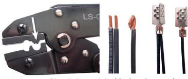
b) Insert the barrel of the connector into the crimping tool so that the "W" of the tool presses on the split side of the barrel. The tool will not release until there is sufficient pressure on the crimp. After crimping, test the wires to be sure they are tight in the connector. If only one wire is to be crimped in the connector, strip 1/2 inch
